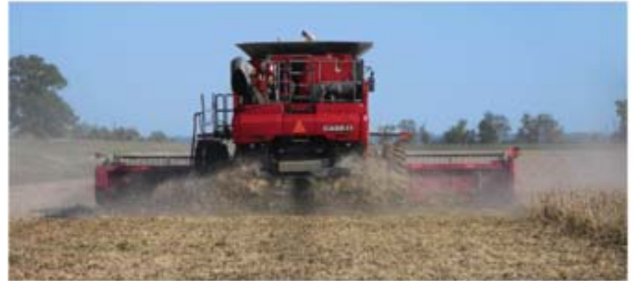
Axial-Flow 8120 spreading residue and chaff.
